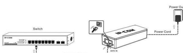
3. Connect one of the AP's RJ45 ports to the PoE adapter's "DATA&PWR OUT" port using a Cat.5 (or higher) twisted-pair cable. (Apart from the AP, it can also be an IP telephone, an IP camera and so on.)
